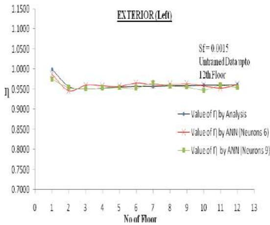
Figure 23. Comparison of obtained value of  $\eta$  from untrained neural network with the actual value obtained from analysis and ANN value (neurons = 6&9) vs. no. of floor for left end (exterior beam)
