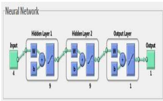
Figure 19. Neural network training with two hidden layer using 9 neurons
