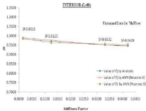
Figure 28. Comparison of obtained value of  $\eta$  from untrained neural network with the actual value obtained from analysis and ANN value (neurons = 6 & 9) vs. stiffness factor for left (interior beam)
