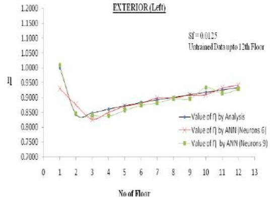
Figure 25. Comparison of obtained value of  $\eta$  from untrained neural network with the actual value obtained from analysis and ANN value (neurons = 6 & 9) vs. no. of floor for left end (exterior beam)
