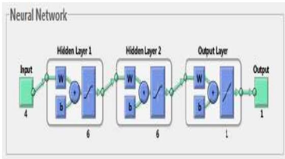
Figure 18. Neural network training with two hidden layer using 6 neurons
