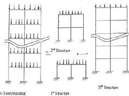
Figure 2. Sequential analysis procedure for N-multi-storey building frame
