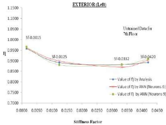
Figure 27. Comparison of obtained value of  $\eta$  from untrained neural network with the actual value obtained from analysis and ANN value (neurons = 6 & 9) vs. stiffness factor for left (exterior beam)
