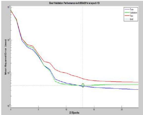
Figure 22. Training graph of exterior beam (right end) with the no. of hidden layer = 2 & no. of neurons = 9
