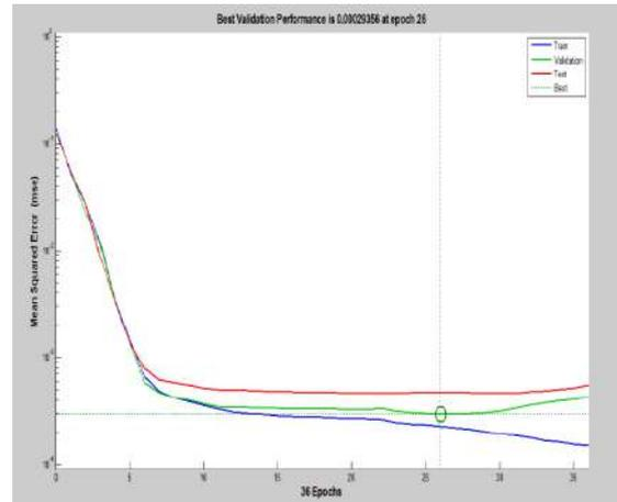
Figure 20. Training graph of exterior beam (left end) with the no. of hidden layer = 2 and no. of neurons = 9
