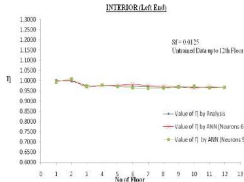
Figure 26. Comparison of obtained value of  $\eta$  from untrained neural network with the actual value obtained from analysis and ANN value (neurons = 6 & 9) vs. no. of floor for left end (interior beam)
