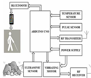
Figure 2. Block diagram of vibrating shoes
